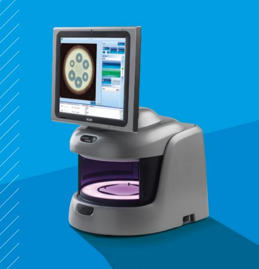
**Protos 3** is an automated colony counter and chromogenic identification system. Using its sensitive CCD camera and unique lighting combined with powerful analysis software, you can count colonies in seconds and automatically identify microbial species by colour on chromogenic plates. You can even use the system with both small and large plates to count colonies on a range of formats including spiral, pour, spread and dilution series plates.
